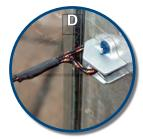
Above are images of the results of LifeLine testing in Canada. As the explosion progresses, you can see in (B) that the sheet of glass has been separated from the frame and is beginning to fold around the shock chords. (C) As the LifeLine cords absorb the blast energy, they effectively prevent the filmed glass from entering the building. (D) Close up of the LifeLine attachment point.
